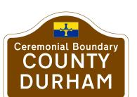
Scale 1:10 Dimensions (mm): Width: 850, Height: 608 x-Heights: 70, 35 Area: 0.45 sq m Colours:
